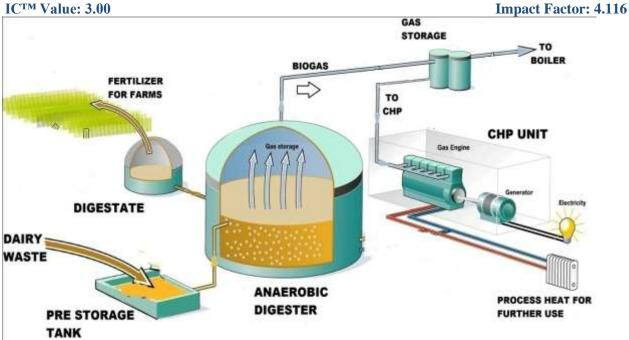
Figure 5 Biogas Plant Layout
