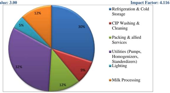
Figure 1 Process Wise Electrical Energy Consumption Profile
