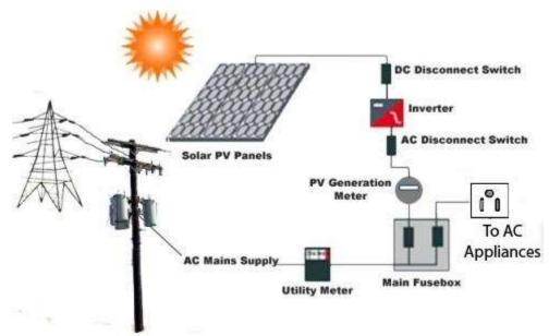
Figure 4 Solar Photovoltaic System Configuration
