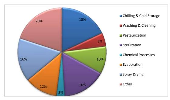
Figure 2 Process Wise Thermal Energy Consumption
